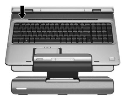
The power status light on the front of the docking station turns on.
