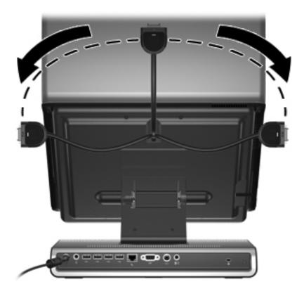
It is important to position the cable correctly, so that the cable can move freely.
