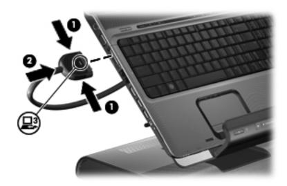
If the computer is already on, the good dock connection light on the expansion cable turns on.
