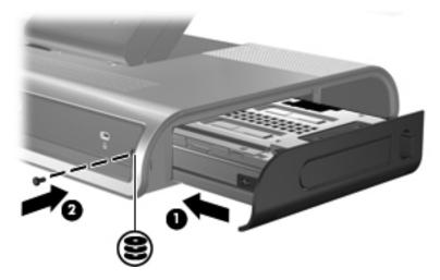
6. Insert the drive **1** into the adapter until the drive is fully seated.
