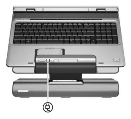
After the computer is docked, the internal computer speakers are disabled and the docking station speakers are activated.
