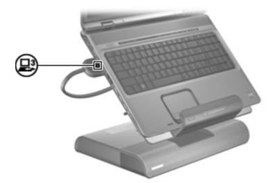
6. If the computer is off, press the power button on the docked computer or the power button on the docking station.
