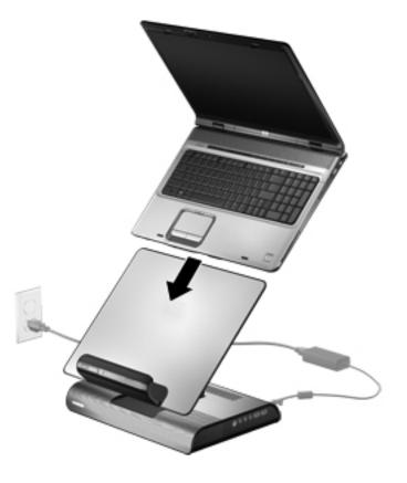
The computer is held in place by a buffer pad, which prevents the computer from shifting out of position.
