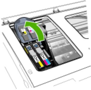
4. Lift the handle of a printhead and use it to pull the printhead out of its slot.
