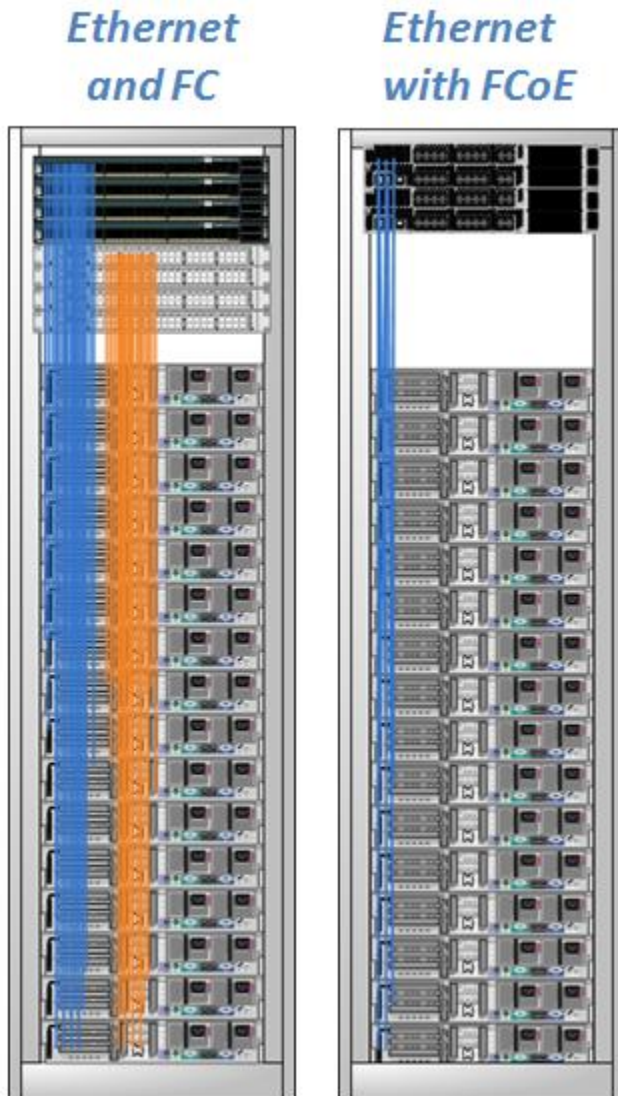
Figure 1 Rack cable comparison
