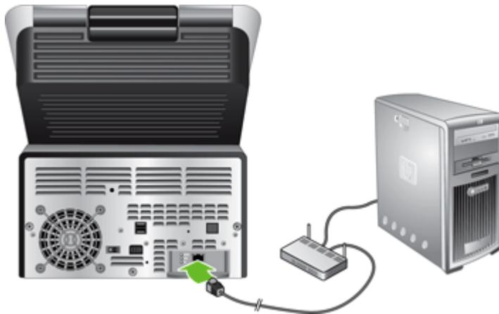
5. Reconnect the power and Ethernet cables, press the Power switch on the back of the product to the on position, and then press the Power button to turn on the product.
