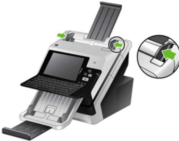
When scanning small originals such as checks, it is especially important that the paper guides fit snugly against the edges of the original.
