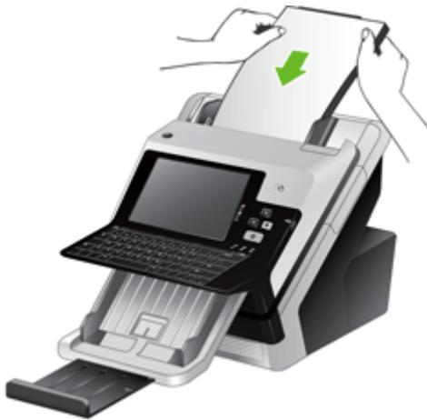
6. Verify that the paper guides are aligned with the edges of the stack.
