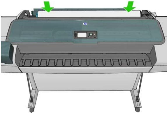
10. If the edge of the roll is not straight or torn (sometimes due to tape used to hold end of the roll), pull the paper slightly and cut a straight edge.
