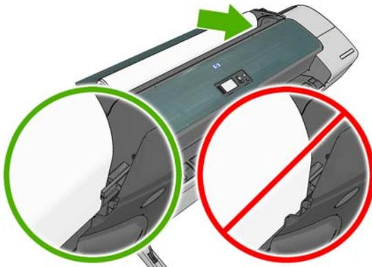
12. Roll the paper into the printer until you feel resistance and the paper flexes slightly. When the printer detects the paper, it feeds it in automatically.
