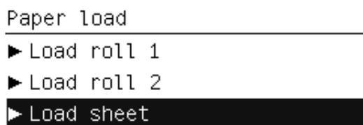
5. If a roll is already loaded, you have to wait while it is automatically unloaded. In the T1200 series only, the roll is not unloaded, but withdrawn to the standby position, so that it can be printed on again without reloading as soon as the sheet paper has been unloaded.
