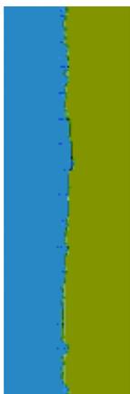
Humidity can cause ink to soak into the paper, making the lines blurred and fuzzy. Try the following:
