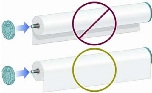
Ensure both ends of the roll are as close to the spindle stops as possible.
