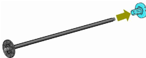
4. If the roll is long; rest the spindle horizontally on a table and load the roll on the table.
