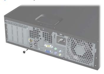
You can now remove the access panel. See Removing the Computer Access Panel on page 4.
