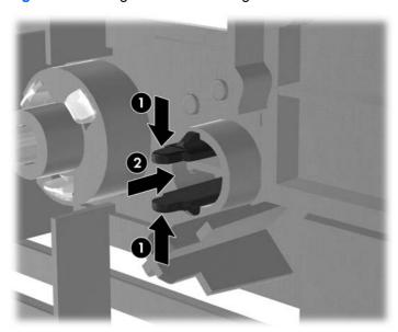
Rotate the HP logo 90 degrees counterclockwise, and then release the logo and press it back into place in the front bezel.
