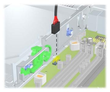
Figure 29 Disconnecting the Media Card Reader 1394 Cable
