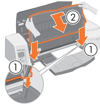
1. Lower the output tray into the printer vertically until it clicks into place and then 2. lower it onto the input tray, sliding the tray slightly to the left may help.
