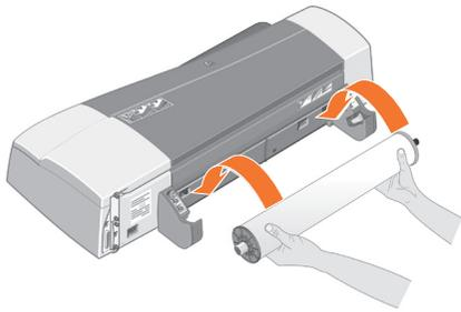
**EN** Insert the spindle into its retaining slots with the blue removable stop on the right and the black stop on the left.
