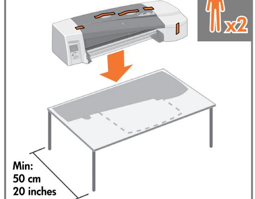
Place the printer on stable surface, respecting the dimensions indicated in the diagram above.
