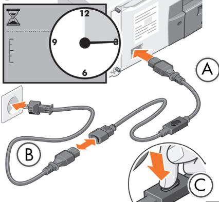
If a short power cable with a switch (A) has been supplied; connect it to the printer, and to the long power cable (B). Otherwise; connect the long cable to the printer (B). Connect the other end to a power socket. Wait 15 seconds. Press the switch (C).
