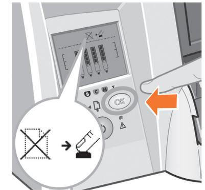
When the two above icons appear; load a single sheet into the front of the printer (see instructions on the printer's cover label), and press the OK Key, or load a roll. The printer will then automatically perform a printhead alignment, and a sheet will be ejected.
