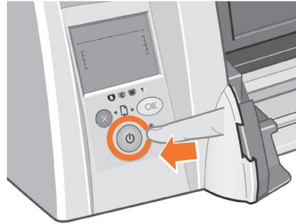
Press the power key to switch the printer on.
