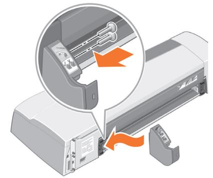
Install the left roll feed assembly, by aligning it with the guides and sliding it into position then using two screws to hold it in place.
