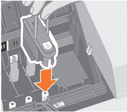
**EN** Match the color of the printhead to the slot in the printer.
