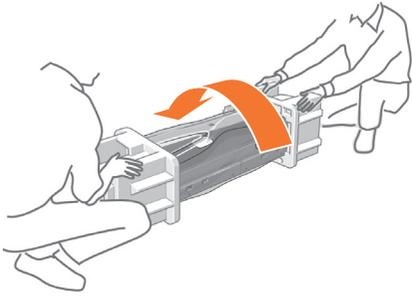
EN Roll the printer into an up right position.
