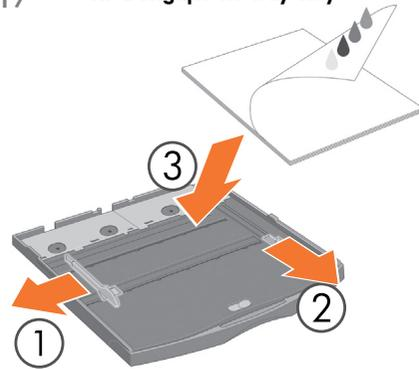
Place the sheets of paper into the corner of the input tray, print side facing down.
