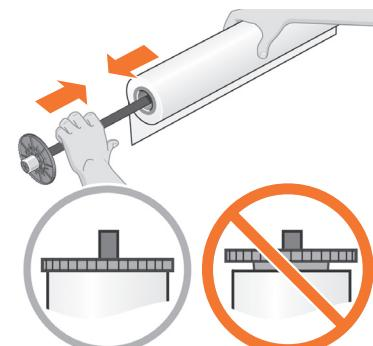
**EN** Insert the spindle into the roll taking care that the leading edge of the roll is on the correct side of the spindle. Ensure the roll is correctly seated as shown above.
