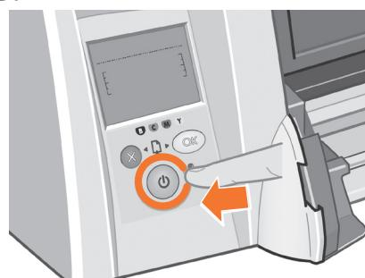
**EN** Press the power key to switch the printer on.
