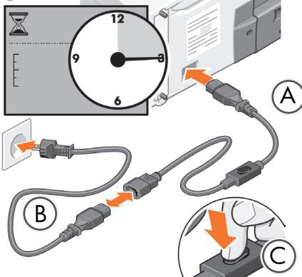
**EN** If a short power cable with a switch (A) has been supplied; connect it to the printer, and to the long power cable (B). Otherwise; connect the long cable to the printer (B). Connect the other end to a power socket. Wait 15 seconds. Press the switch (C).
