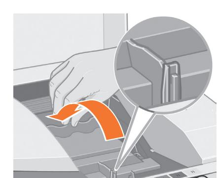
Return the printhead cover to its original position ensuring that the hook and the latch engage.
