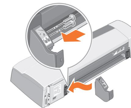
**EN** Install the left roll feed assembly, by aligning it with the guides and sliding it into position then using two screws to hold it in place.
