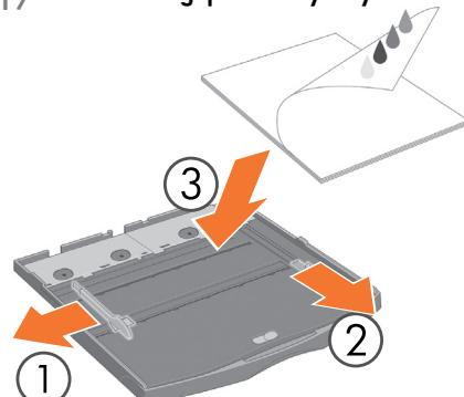
**EN** Place the sheets of paper into the corner of the input tray, print side facing down.
