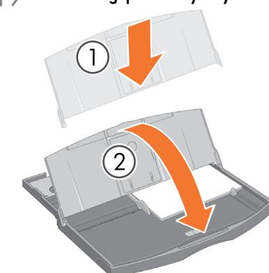
**EN** Locate the dust cover and insert it into the input tray from above and lower it down.
