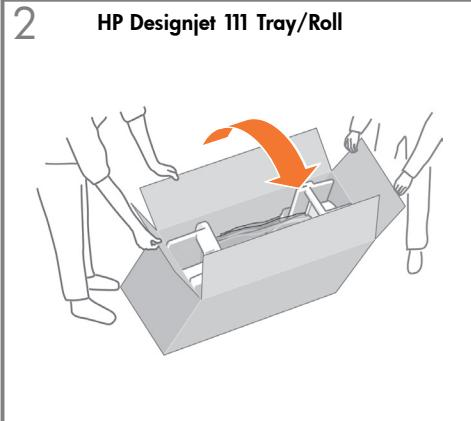
**EN** Roll the box onto its side. Note: If you have an HP Designjet 111 Roll, make sure you remove the spindle before you roll the box.
