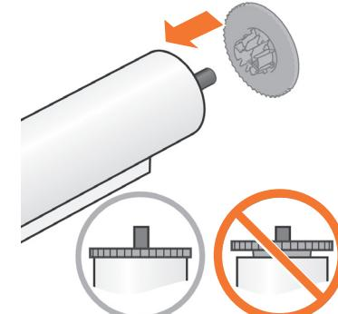
**EN** Insert the blue removable stop onto the spindle. Ensure it is correctly seated as shown above.
