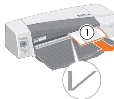
When the sand clock icon disappears the printer will automatically perform a printhead alignment and a sheet (1) will be ejected.
