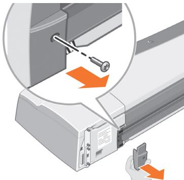
**EN** Remove the left plastic insert by extracting the screw as shown.
