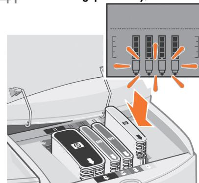
**EN** When the last ink cartridge is inserted only the printhead icons should be flashing.
