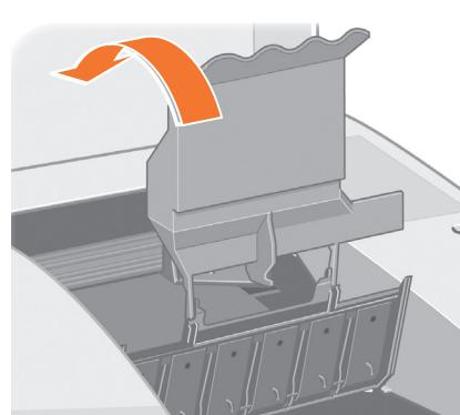
**EN** Lift the whole printhead cover back so that the printhead slots are exposed.
