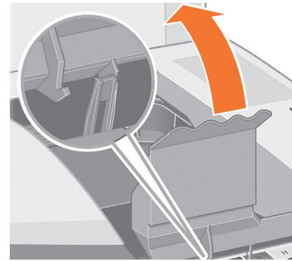
**EN** The hook at the front should unlatch itself. Lift the printhead cover back.
