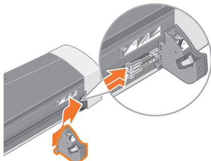
**EN** Install the right roll feed assembly, by aligning it with the guides and sliding it into position then using two screws to hold it in place. You may have a screw left over after assembly has been completed.
