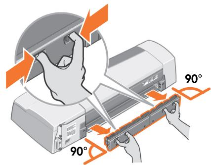
**EN** Remove the rear path by pressing the buttons as shown, and carefully pulling it straight out.
