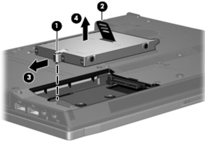
7. If it is necessary to replace the hard drive bracket, remove the two Phillips PM3.0x4.0 hard drive bracket screws **(1)** from each side of the hard drive.
