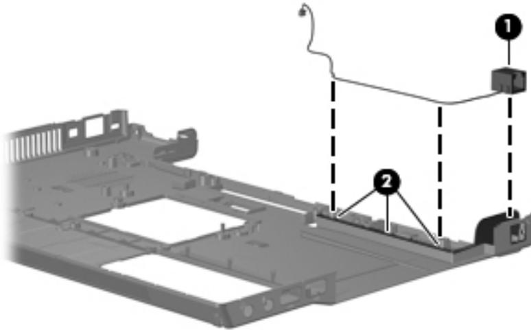
3. Remove the RJ-11 connector cable from the base enclosure.
