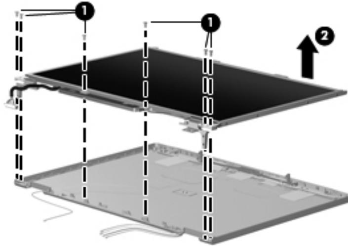
12. Remove the four Phillips PM2.0x4.0 screws **(1)** that secure each display hinge to the display panel.
