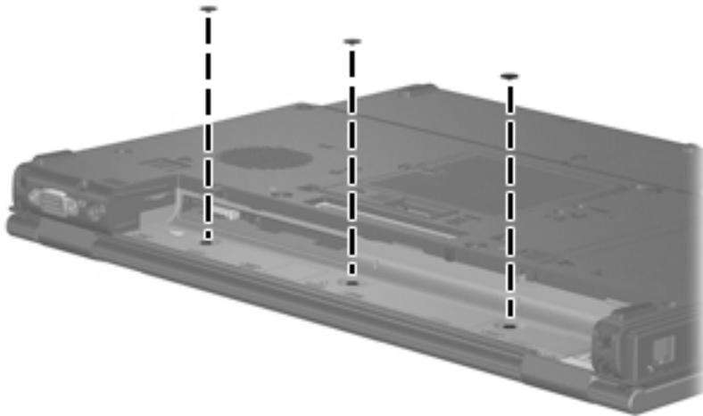
**Where used:** 3 screws that secure the switch cover to the computer
