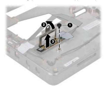
Reverse this procedure to install the Fingerprint reader board assembly.
