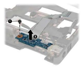
Reverse this procedure to install the Wireless/web/mute function board assembly.
