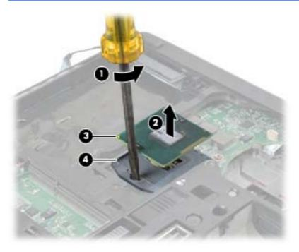
Reverse this procedure to install the processor.
