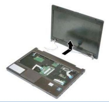
CAUTION: When installing the display assembly, be sure that the wireless antenna cables routed out of the display right hinge are routed and arranged properly.
