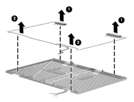
19. If it is necessary to remove the WLAN antenna transceivers (1) and cables, remove them from the display enclosure back cover by lifting them (2) from the clips in the display enclosure back cover.
