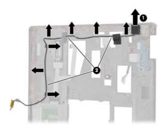
Remove the RJ-11 connector cable from the top cover.
