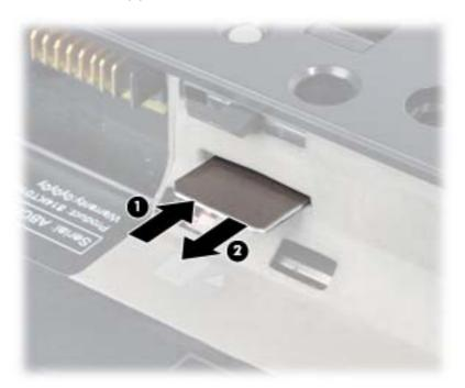
Reverse this procedure to install the SIM.
