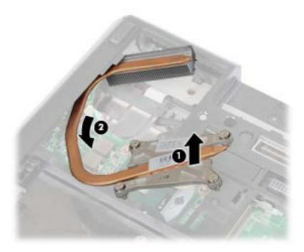
NOTE: The thermal material must be thoroughly cleaned from the surfaces of the heat sink (1) each time the heat sink is removed. Thermal material is included with all heat sink and processor spare part kits.
