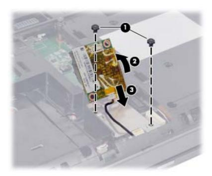
Reverse this procedure to install the modem module.
