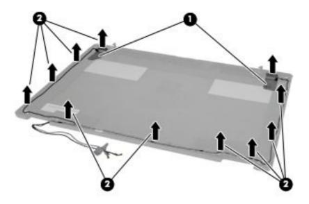
20. If it is necessary to replace the display panel hinges, remove the six Phillips PM2.0×3.0 screws (1) that secure the display panel hinges to the display panel, three screws on the left and three screws on the right.
