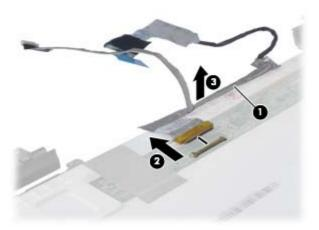
17. If it is necessary to replace the display hinges, remove the six Phillips PM2.5×3.0 screws (1) that secure each display hinge to the display panel.
