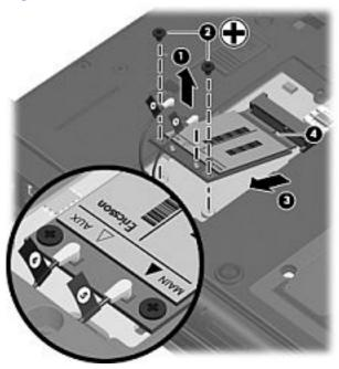
Figure 4-2 Qualcomm module antenna locations
