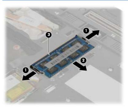
Reverse this procedure to install an expansion memory module.
