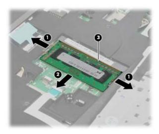
Reverse this procedure to install a primary memory module.
