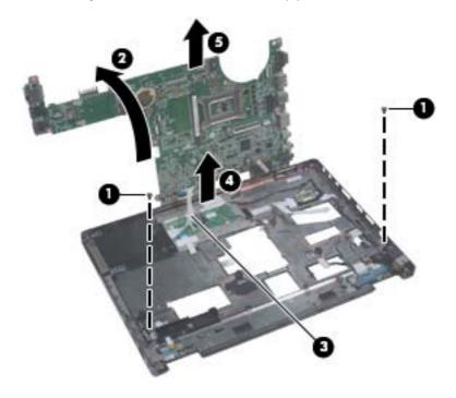
Reverse the preceding procedure to install the system board.
