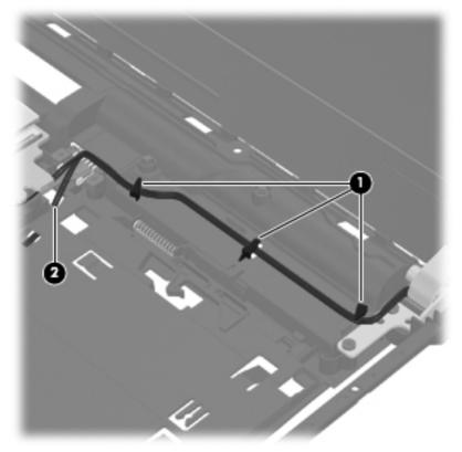
Cable routing path – bottom
