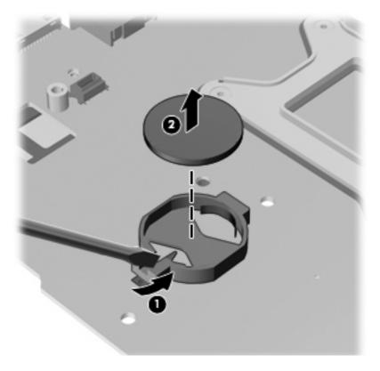
Reverse this procedure to install the RTC battery.
