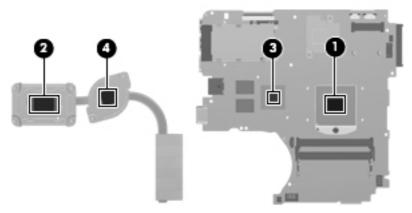
NOTE: For UMA models, thoroughly clean thermal material from the surface of the system board (1) and heat sink (2) each time you remove the heat sink. All heat sink and processor spare part kits include thermal material.
