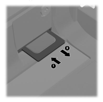
Reverse this procedure to install the SIM.
