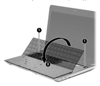
**9.** Lift the keyboard connector latch **(1)**, and then disconnect the keyboard cable from the system board **(2)**.
