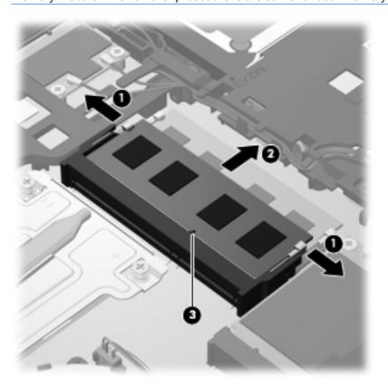
Reverse this procedure to install a memory module.
