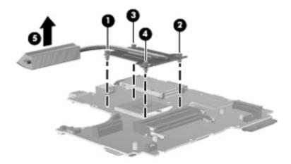
NOTE: For discrete models, thoroughly clean thermal material from the surfaces of the system board components (1)(3) and the heat sink (2)(4) each time you remove the heat sink. All heat sink and processor spare part kits include thermal material.
