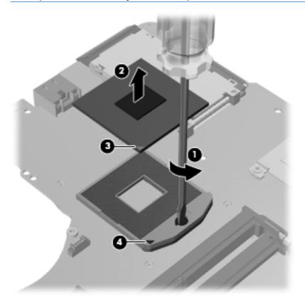
Reverse this procedure to install the processor.
