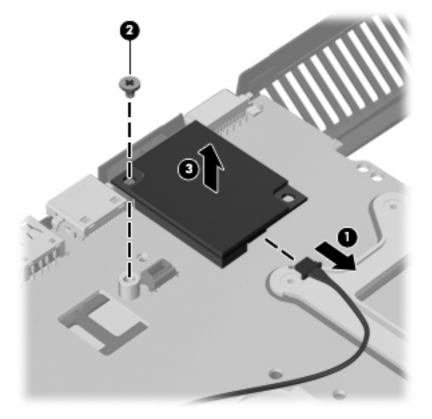
Reverse this procedure to install the modem module.
