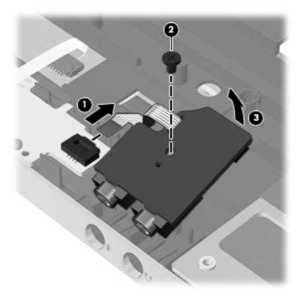
Reverse this procedure to install the audio board.
