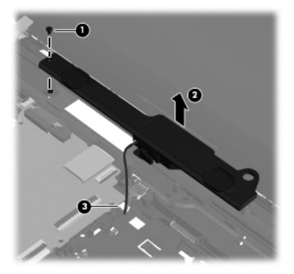
Reverse this procedure to install the speaker assembly.
