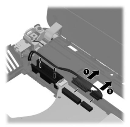
Remove the two Phillips PM2.5×4.0 screws (1) that secure the security bracket to the computer, and then lift the security bracket from the computer (2).
