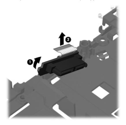
Reverse this procedure to install the optical drive connector.
