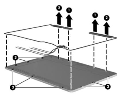
A CAUTION: When installing the display assembly, be sure that the wireless antenna cables are routed and arranged properly.
