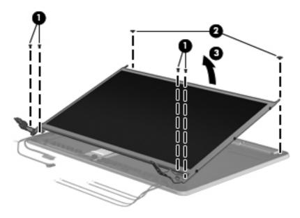
14. Disconnect the display panel cable from the back of the display panel by lifting the tape over the connector (1), and then disconnecting the cable from the panel (2).
