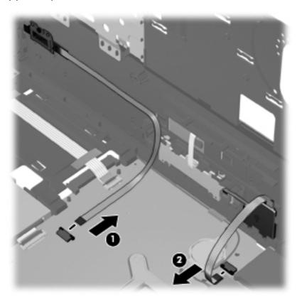
6. Disconnect the Quick Launch board cable from the system board.
