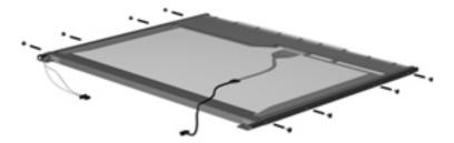
Use a sharp-edged tool to cut the tape (1) that secures the sides of the display panel to the display panel frame.
