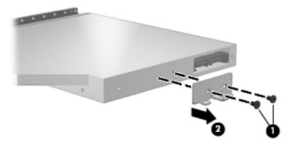
Reverse this procedure to install an optical drive.
