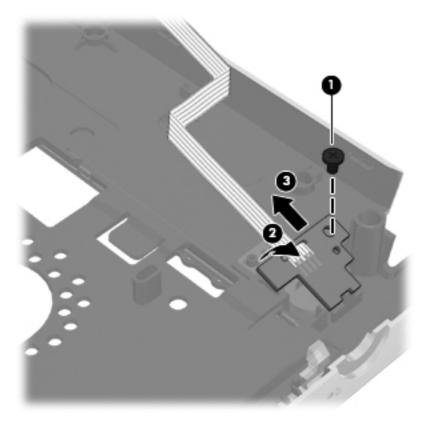
Reverse this procedure to install the Quick Launch board.
