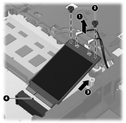
NOTE: If the WWAN antennas are not connected to the terminals on the WWAN module, the protective sleeves must be installed on the antenna connectors, as shown in the following illustration.
