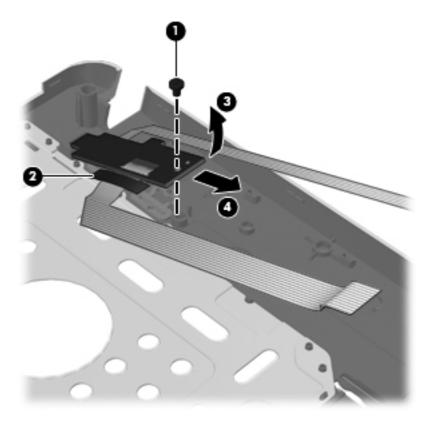
**5.** Remove the Phillips PM2.0×3.0 screw **(1)** that secures the board to the top cover.
