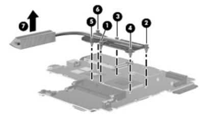
To remove the UMA heat sink, in the order indicated, loosen the four captive Phillips screws (1)
