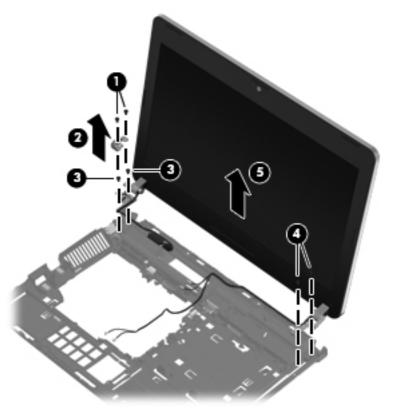
(CAUTION: When installing the display assembly, be sure that the wireless antenna cables are routed and arranged properly.
