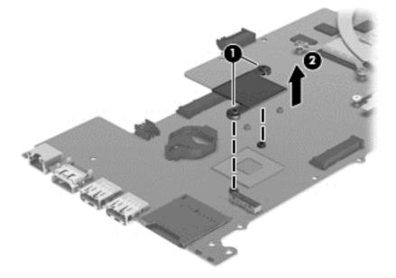
Reverse this procedure to install the PCH heat sink onto a replacement system board.
