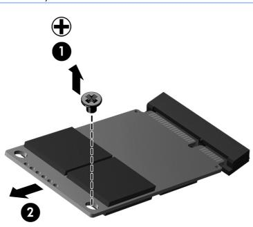
Reverse this procedure to install the mSATA drive onto a replacement system board.
