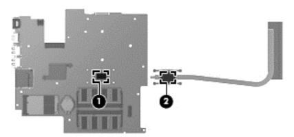
**3.** Reverse this procedure to replace the heat sink. Replace the thermal material that ships with the replacement heat sink.
