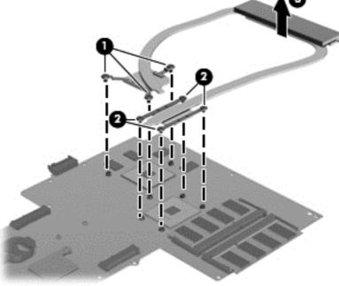
b. Thoroughly clean the thermal connections (1), (3) on the system board and the heat sink (2), (4) before replacing a heat sink onto a system board. Continue to step 3.
