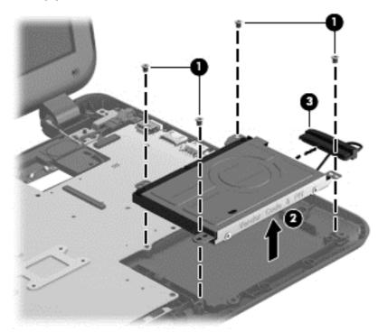
3. Remove the four Phillips screws (1), and then remove the bracket (2) from the hard drive.
