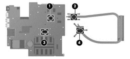
c. Loosen the captive screws (1) and lift the UMA graphics heat sink (2) from the system board.
