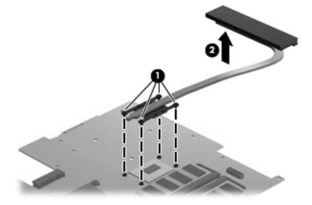
**d.** Thoroughly clean the thermal connections (1) on the system board and the heat sink (2) before replacing a heat sink onto a system board.
