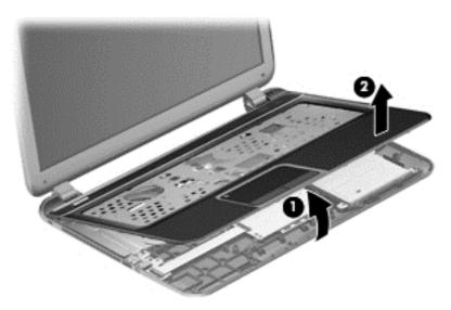
When replacing the top cover, be sure that the following components are removed from the defective top cover and installed on the replacement top cover:
