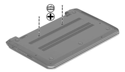
2. Turn the computer right-side up with the front toward you. Open the display and stand the computer on its right side. Insert a thin tool through the keyboard access hole. (The keyboard icon indicates the keyboard access hole.) Push firmly on the bottom of the keyboard until it disengages from the computer.
