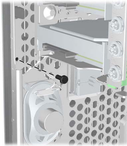
Figure 6-4 Installing the Front Bezel Security Screw
