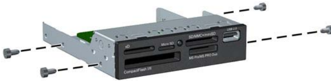
Figure 7-21 Installing Guide Screws (Media Card Reader Shown)
