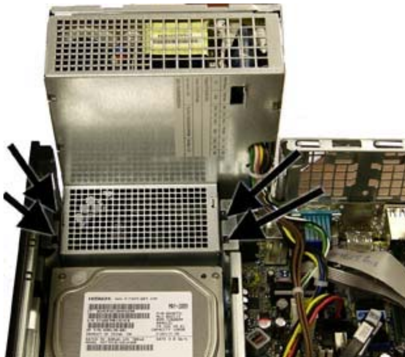
Figure 7-47 Removing the power supply
