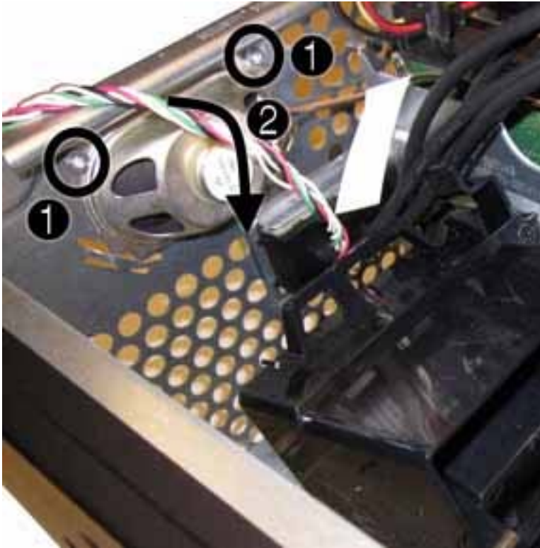
Figure 6-41 Removing the speaker
