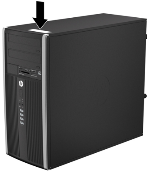
Figure 1-7 Small Form Factor Serial Number and Product ID Location
