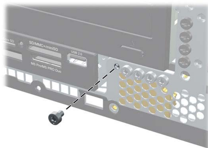
Figure 7-3 Retrieving the Front Bezel Security Screw
