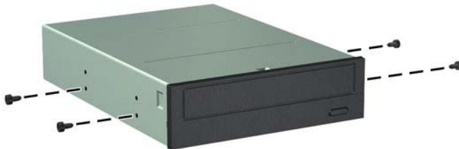
Figure 6-18 Installing Guide Screws (Optical Drive Shown)
