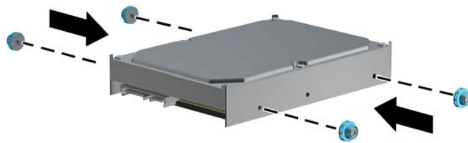
Figure 6-23 Installing Isolation Mounting Guide Screws in a 3.5-inch Drive
