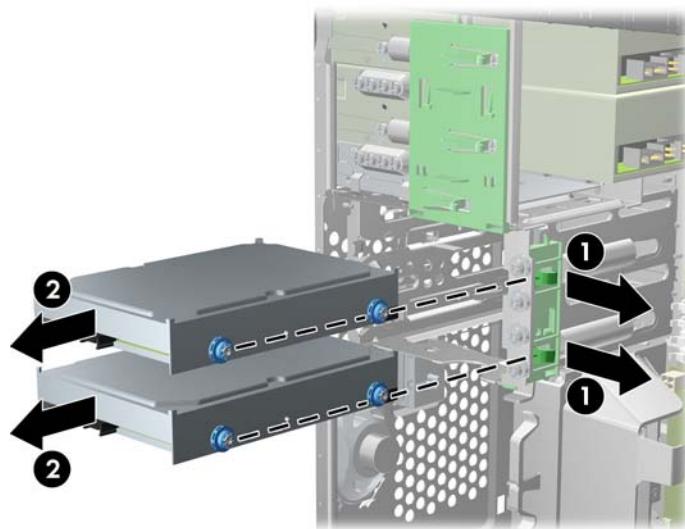
Figure 6-22 Removing a Hard Drive
