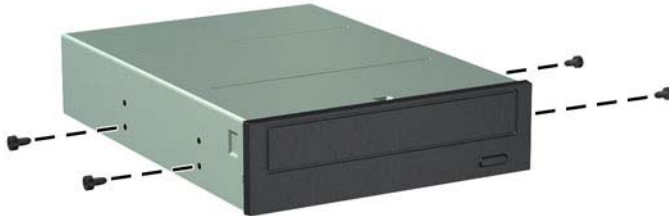
Figure 7-17 Installing Guide Screws in the Optical Drive
