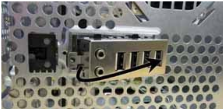
Figure 6-39 Removing the front I/O assembly
