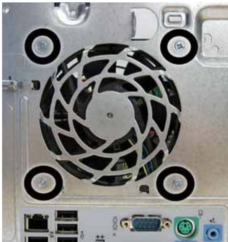
Figure 6-42 Rear fan screws
