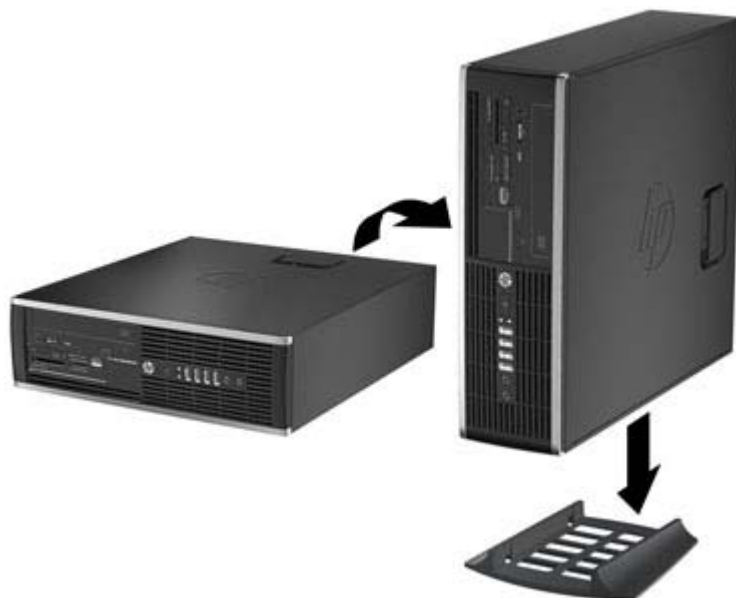
Figure 7-49 Changing from Desktop to Tower Orientation
