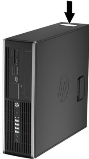
Figure 1-7 Small Form Factor Serial Number and Product ID Location
