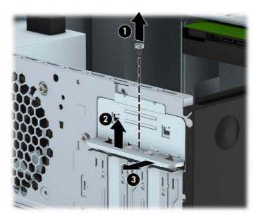
Locate the correct vacant expansion socket on the system board and the corresponding expansion slot on the back of the computer chassis.
