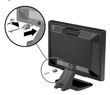
3. Slide the security cable through the hole in the cable lock on the rear of the monitor.
