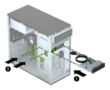
8. If installing a USB 3.0 media card reader, connect the media card reader 3.0 cable to the USB 3.0 to USB 2.0 adapter (1) and connect the adapter to the connector on the system board labeled MEDIA (2).
