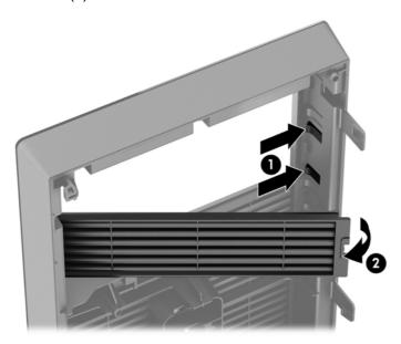
• To remove a 3.5-inch bezel blank, press inward on the two retaining tabs on the side of the bezel blank that hold the bezel blank in place (1) and rotate the bezel blank back to remove it (2).
