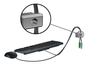
Screw the lock to the chassis using the screw provided. 6.
