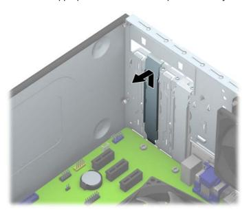
**b.** If you are removing a PCI Express x1 card, hold the card at each end and carefully rock it back and forth until the connectors pull free from the socket. Lift the card straight up (1) then away from the inside of the chassis (2) to remove it. Be sure not to scrape the card against other components.
