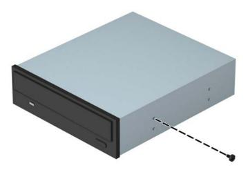
8. Slide the drive into the drive bay (1) and install the two M3 mounting screws in the side of the drive (2) to secure it in place.
