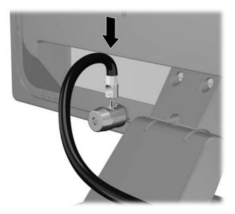
4. Use the bracket provided in the kit to secure other peripheral devices by laying the device cable across the center of the bracket (1) and inserting the security cable through one of the two holes in the bracket (2). Use the hole in the bracket that best secures the peripheral device cable.
