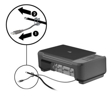
Thread the keyboard and mouse cables through the computer chassis lock.
