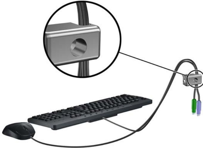
6. Screw the lock to the chassis using the screw provided.
