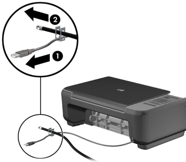
5. Thread the keyboard and mouse cables through the computer chassis lock.
