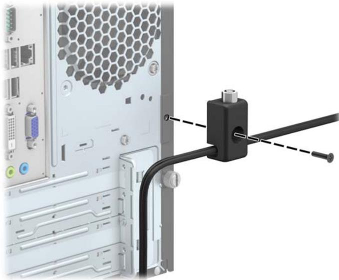
7. Insert the plug end of the security cable into the lock (1) and push the button in (2) to engage the lock. Use the key provided to disengage the lock.
