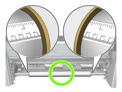
Some lower-quality rolls may be poorly wound onto the cores during manufacturing, resulting in skew and telescoping during printing. This may lead to smears and other image quality issues. The maximum tolerated skew or telescoping according to Latex 3000 printer specifications is 5mm (0.197 in).
