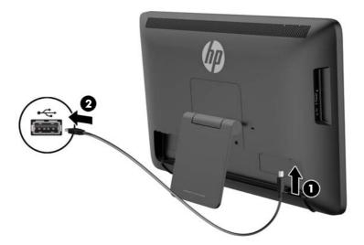
7. Connect one end of the power cord to the AC power connector on the back of the all-in-one (1), route the cord through the retainer clip (2), and then connect the other end to an electrical wall outlet (3).
