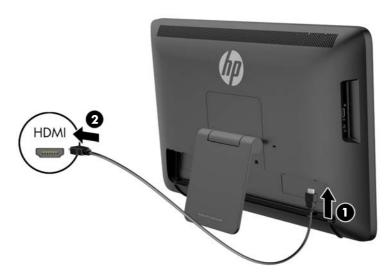
6. If you want to use the keyboard and mouse in HDMI mode or provide touch functionality to the screen while connected to a PC in HDMI mode, connect a USB cable to the USB upstream port on the rear panel of the all-in-one (1), and then to a USB downstream port on the PC (2).
