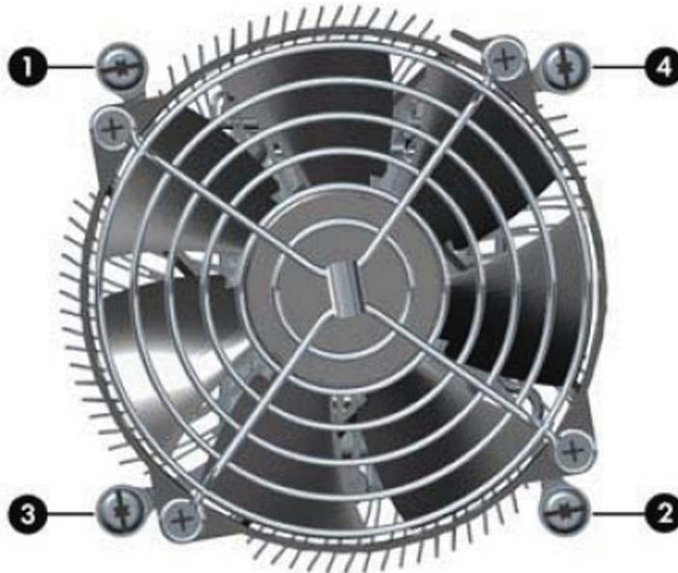
Figure 6-44 Loosening the fan sink screws
