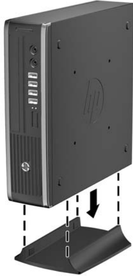
Figure 9-34 Placing the computer on the stand
