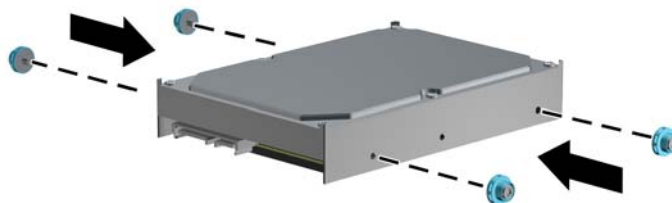
Figure 7-21 Installing Isolation Mounting Guide Screws in a 3.5-inch Drive
