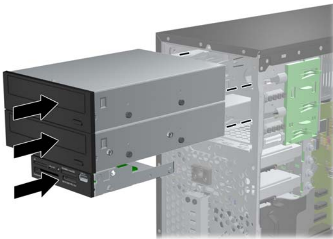
Figure 7-18 Sliding the Drives into the Drive Cage
