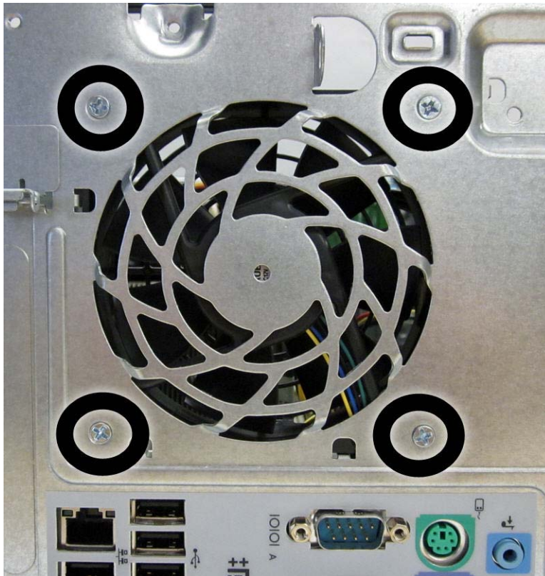
Figure 7-32 Rear fan screws
