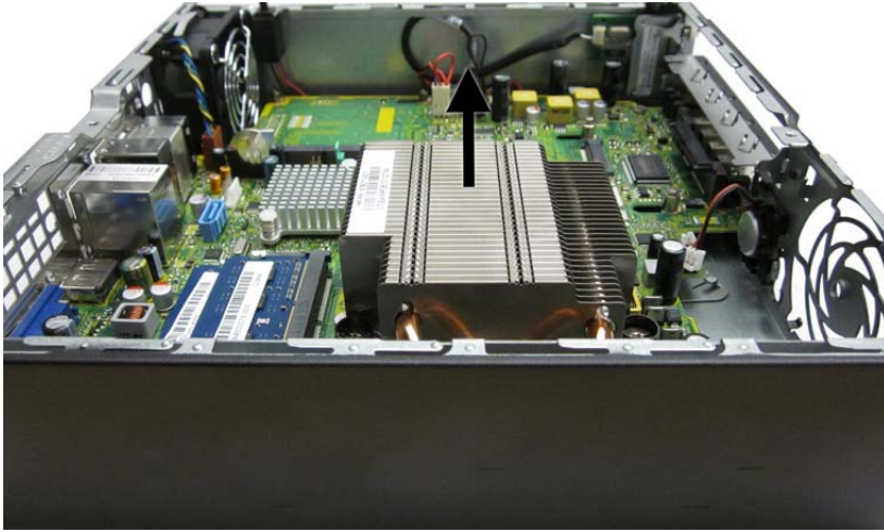
Figure 9-24 Removing the heat sink
