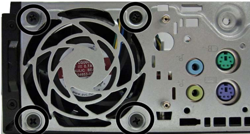
Figure 9-32 Removing the rear fan screws
