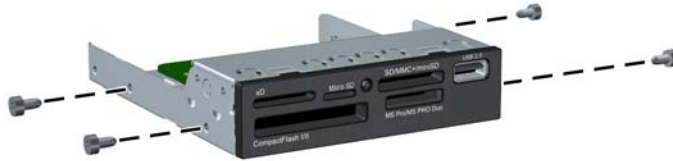
Figure 8-20 Installing Guide Screws (Media Card Reader Shown)
