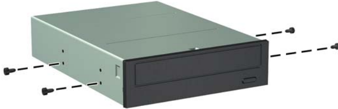
Figure 7-17 Installing Guide Screws (Optical Drive Shown)
