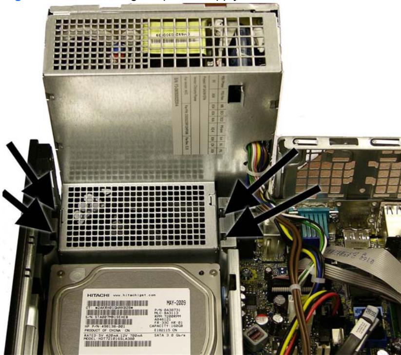
Figure 8-38 Removing the power supply
