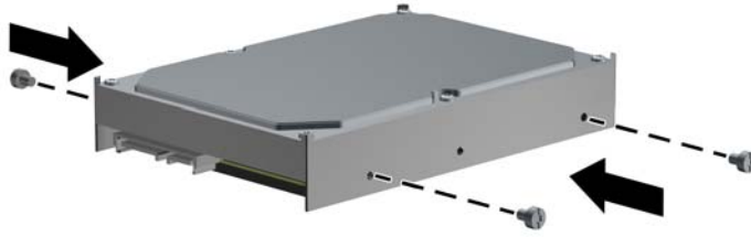
Figure 6-26 Installing Standard Guide Screws
