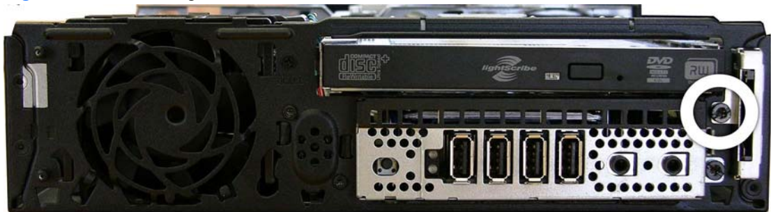
Figure 9-20 Removing the card reader screw
