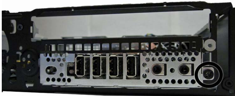
Figure 9-29 I/O panel screw
