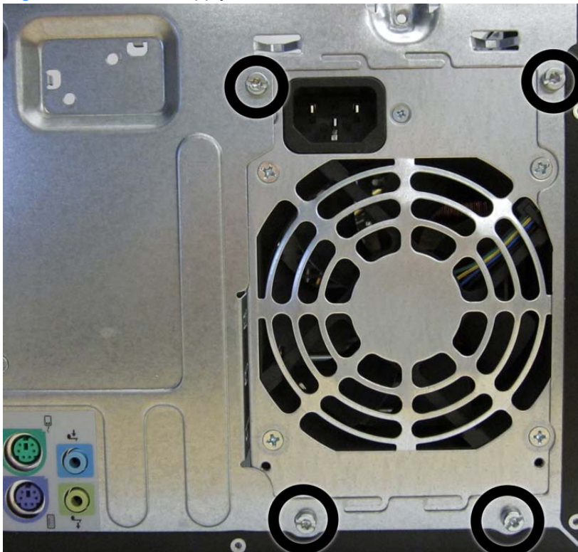
Figure 7-34 Power supply screws
