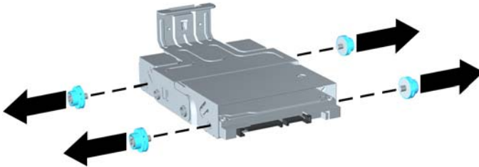
Figure 9-14 Removing the guide screws
