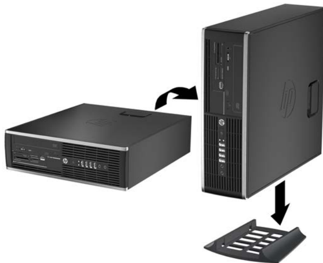
Figure 8-40 Changing from Desktop to Tower Orientation
