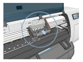
5. Pull up and release the latch on top of the carriage.
