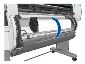
**18.** If the paper that you are using has a barcode printed on the leading edge of the roll, and **Printing paper info** is enabled, the printer automatically reads the information.
