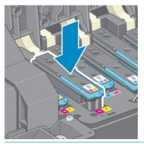
▲ CAUTION: You might feel some resistance when installing the new printhead, so you need to press it down firmly but smoothly. You should hear a beep and see confirmation on the front-panel display that the printhead has been inserted. If you have difficulty, see <u>Cannot insert a printhead on page 158</u>.
