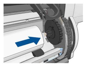
**10.** Push the left hub onto the left end of the roll, by pressing the stopper (blue lever). Check that the hub disc is aligned with the green mark.
