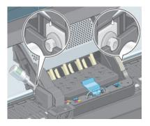
4. Apply a few drops of oil directly to the slider rod on either side of the carriage.
