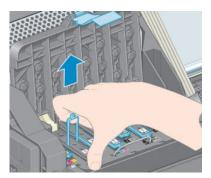
9. Gently pull the blue handle upward until the printhead is released from the carriage.
