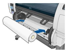
9. Insert the right side of the roll onto the right hub. Check that the roll is in contact with the disc.
