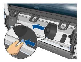
8. Put the roll into the cavity with the paper edge on the near side facing downwards.
