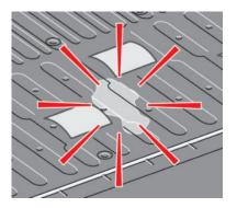
5. If oil spills onto the platen, wipe the platen clean by using the cloth that was supplied with the maintenance kit.
