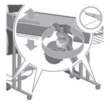
3. When the correct height has been achieved, tighten the upper hexagonal nut.
