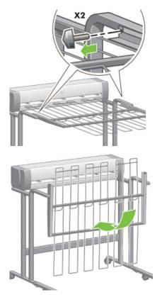
2. Remove the pin from each leg extension, and rotate the leg extension upwards.
