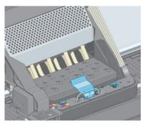
When all of the printheads have been inserted correctly and the printer has accepted them, the printer beeps.
