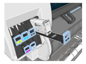
**5.** Lift the cartridge out of its drawer.
