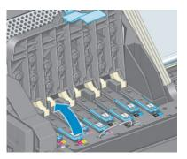
8. Using the blue handle, gently disengage the printhead.
