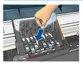
3. Rub the cloth against the electrical contacts with a *light* force along the entire depth of the flex connector. Try to avoid picking up any ink deposit that may have accumulated on the bottom surface of the slot.
