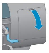
3. The maintenance cartridge has a handle on the front. To remove the cartridge, press inward and upward as indicated by the arrow, until the cartridge is released.
