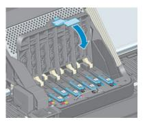
6. Make sure that the end of the blue handle catches the wire loop on the near side of the carriage.
