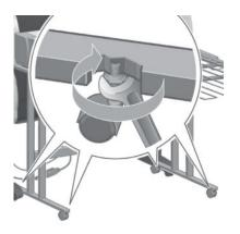
2. Adjust the height of the stacker by rotating the lower hexagonal nut clockwise or anti-clockwise.
