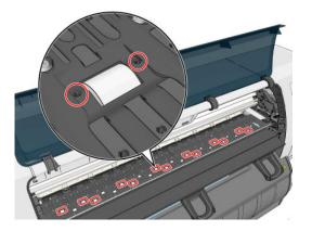
4. Put three drops of oil into each hole in the platen.
