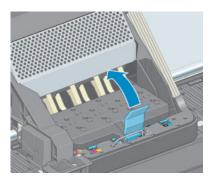
7. To remove a printhead, lift up the blue handle.
