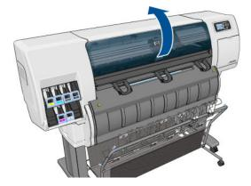
5. Find the printhead drop detector to the right of the printhead carriage.
