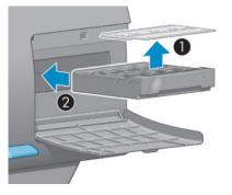
2. When the maintenance cartridge has been pushed all the way in, press inwards and downwards as indicated, until it clicks into place.
