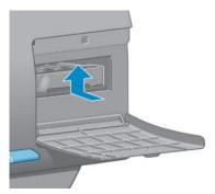
4. Lift up the maintenance cartridge to remove it from the slot, and slide it out.
