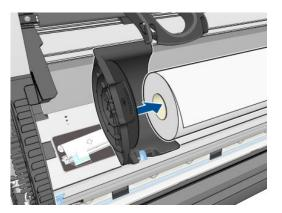
**11.** Check that there is no gap between the roll and either of the hubs.
