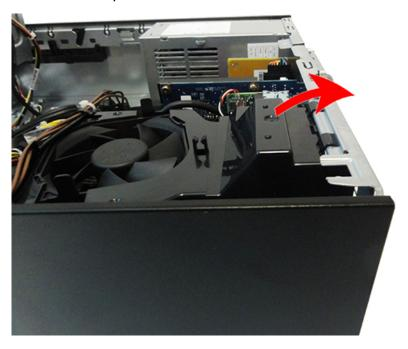
Pull the baffle away from the rear of the computer to disengage the clips on the baffle from the rear of the computer.
