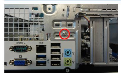
4. From the inside of the computer, lift the hood lock out of the computer..
