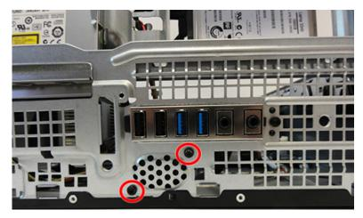
6. From the inside of the chassis, disconnect the speaker cable from the white system board labeled SPKR, and the remove the speaker from the chassis.
