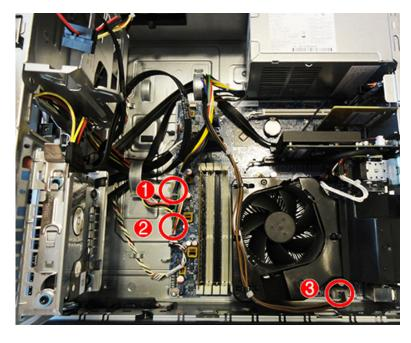
5. From the outside, rear of the chassis, remove the three Torx T15 that secure the power supply to the back of the chassis.
