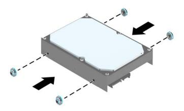
6. Align the mounting screws with the slots on the chassis drive cage, press the hard drive down into the bay, and then slide it forward until it stops and locks in place.
