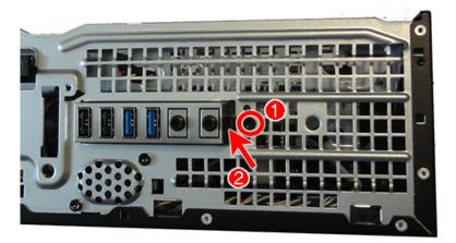
9. Remove the front I/O assembly from the inside of the computer.
