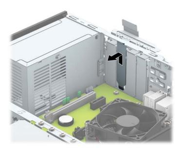
**b.** If you are removing a PCI Express x1 card, hold the card at each end, and carefully rock it back and forth until the connectors pull free from the socket. Pull the expansion card straight up from the socket (1) then away from the inside of the chassis to release it from the chassis frame (2). Be sure not to scrape the card against the other components.
