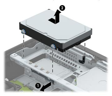
5. To install a hard drive, you must transfer the mounting screws from the old hard drive to the new hard drive.
