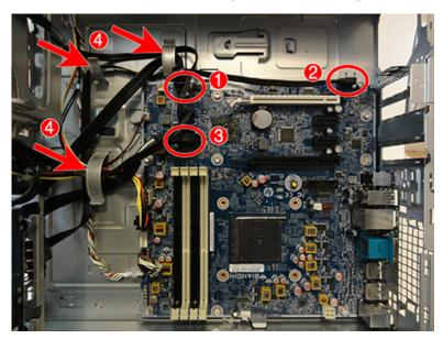
**7.** Remove the Torx T15 screw **(1)** that secures the assembly to the front of the chassis.
