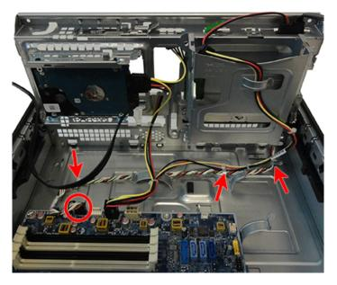
7. Remove the power switch assembly from the inside of the computer.
