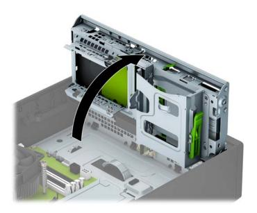
5. Align the mounting screws on the drive with the J-slots on the sides of the drive bay. Press the drive up into the drive bay then slide it forward until it locks in place.
