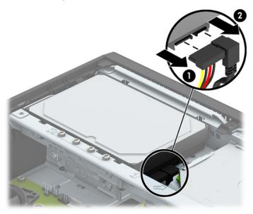
4. Pull the release lever next to the rear of the hard drive outward (1). While pulling the release lever out, slide the drive back until it stops, and then lift the drive up and out of the bay (2).
