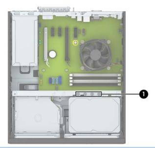
NOTE: You can also use one of the extra mounting screws to secure the front bezel (see Front bezel security on page 21 for more information).
