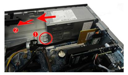
To install the power supply, reverse the removal procedure.
