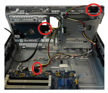
To reinstall the drive power cable, reverse the removal procedure.
