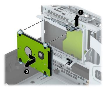
6. If you are installing a new drive, refer to <u>Installing a 2.5-inch hard drive on page 43</u>. If you are not installing a new drive, rotate the drive cage down and replace the access panel.
