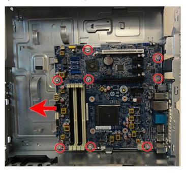
When reinstalling the system board, first insert the I/O panel back into the slots in the rear of the chassis, and then align the board with the chassis screw holes.
