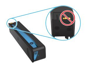
6. Insert the new cartridge into the product. Make sure the cartridge is firmly in place.
