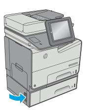
Pull the tray completely out of the printer by pulling and lifting it up slightly.
