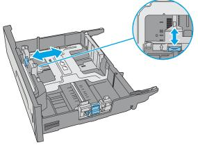
4. Load paper into the tray. Check the paper to verify the guides lightly touch the stack, but do not bend it. For information about how to orient the paper, see 3 x 500-sheet tray paper orientation on page 32.
