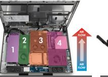
The system layout was designed for quiet acoustics in the same way all HP Z workstations are. Cool air enters the bottom of the system and is directed upward through the four independent thermal zones. The zones are:
