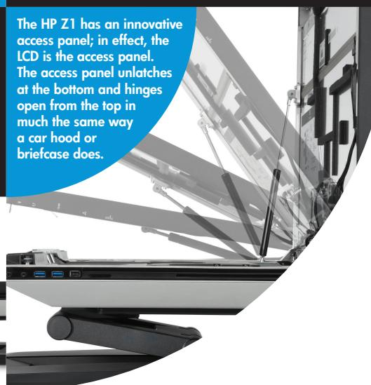
The HP Z1 has an innovative access panel; in effect, the LCD is the access panel. The access panel unlatches at the bottom and hinges open from the top in much the same way a car hood or briefcase does.
