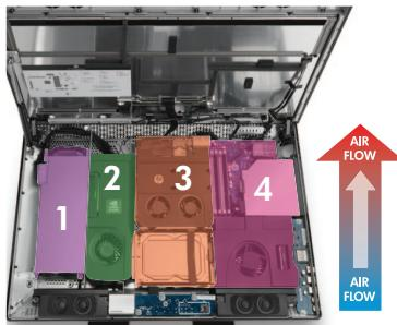
The system layout was designed for quiet acoustics in the same way all HP Z workstations are. Cool air enters the bottom of the system and is directed upward through the four independent thermal zones. The zones are:
