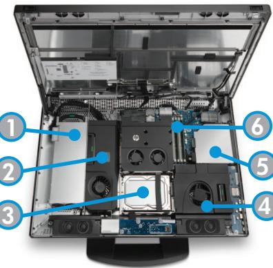
Similar to other HP Z Workstations, the HP Z1's internal components are easily serviceable, and most of them require no tools to remove and replace. The following components are all tool-less:
