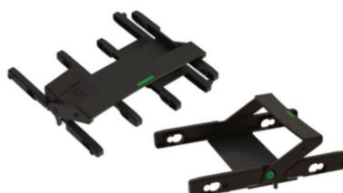
Hard drives are secured in the HP Z1 with easy to use hard disk drive carriers that have tool-less installation of 1 x 3.5" disk or 2 x 2.5" disks. These options use different carriers, but both allow the same degree of serviceability and ease of use. Elastomeric dampers are integrated into these carriers to prevent the drives from transmitting noises into the system, and the system from transferring vibrations into the drives reducing their performance.
