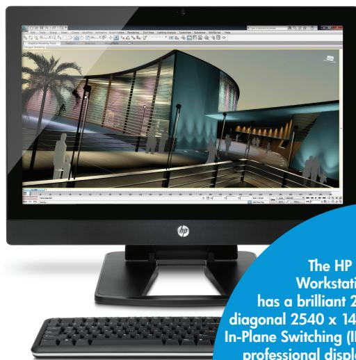
The HP Z1 Workstation has a brilliant 27" diagonal 2540 x 1440 In-Plane Switching (IPS) professional display.
