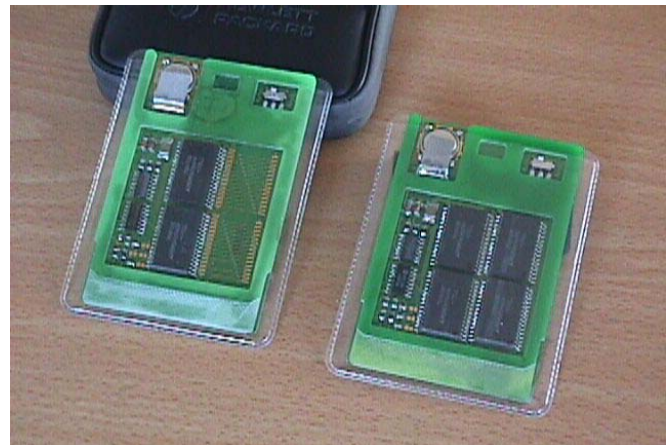
Fig. 10 - Homebrew RAM-memory plug-in cards for the HP48 series calculators at the HPCC1997 conference in London.
