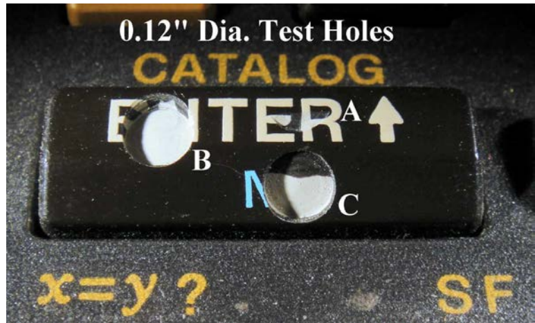
Fig. 1 – Three holes “drilled” into HP-41C ENTER Key,
