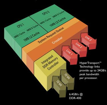
AMD is continuing to drive technology leadership by introducing another computing first: multi-core technology for the x86-based computing market. Dual-core AMD Opteron processors for servers and workstations extend AMD's Direct Connect Architecture by connecting two CPUs on one die, improving overall system performance and efficiency.
