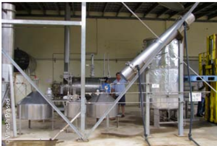
Steam distillery apparatus for sandalwood oil at Tropical Rainforest Aromatics, Vanuatu.
