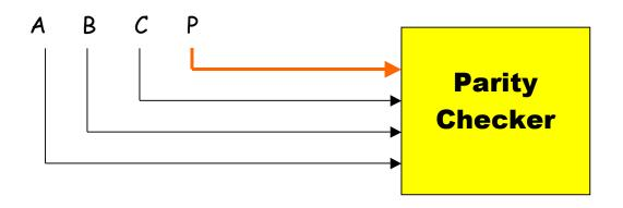
The parity-bit generator generates a P so that the number of 1's in the transmitted data is odd (or even). The **parity checker** checks this in the received data. How will you design (1) a parity-bit generator, and (2) a parity checker?
