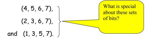
The receiver, upon receiving the 7-bit data, computes the parities of the above bit combinations, and reports the result using three bits b2, b1, b0 as follows:
