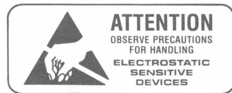
Figure 5. Approved label for electrostatic sensitive devices.
