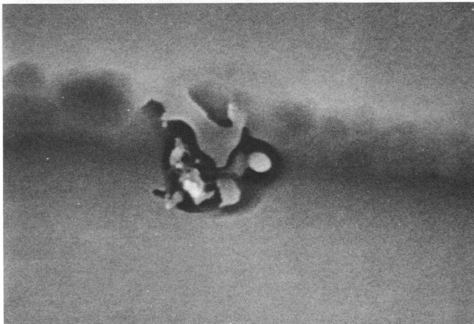
Figure 2. This is a blowup (23,000X) of one of the craters shown in Figure 1. The crater is ~1 micron wide and contains fragments of melted metal.
