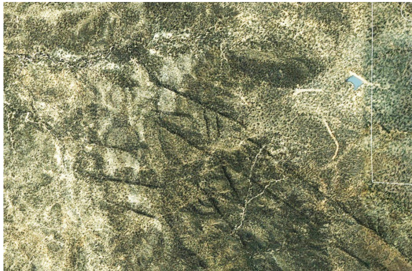
Figure 29 - Joints and Faulting at the Northern Terminus of the Magnetic Anomaly. (After Google Map – Lineaments Emphasized)
