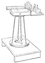
inch shorter. The common length of the English glass slides being three inches, the stage must be five inches wide, to admit of their moving about freely. From these dimensions several of the others are naturally derived.
