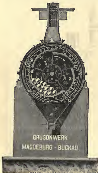
Fig. 11.—Transverse Section of Ball-mill.
