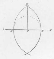
Answer.—From the given point C as centre describe an arc so as to cut the line A B in two points D and E. From the points D, E, with a radius equal to D E, describe arcs cutting each other at F, draw the straight line F C, then F C is perpendicular to A B and A C F is a right angle = to | \( \textstyle \).
