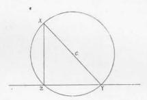
any line X Y from the given point to the given line at an angle about  $45^{\circ}$ — $60^{\circ}$ : bisect this line and from the centre C draw a circle passing through the point and then join it to the point Z where this circle cut the original line—then X Z is at right angles to Z Y.
