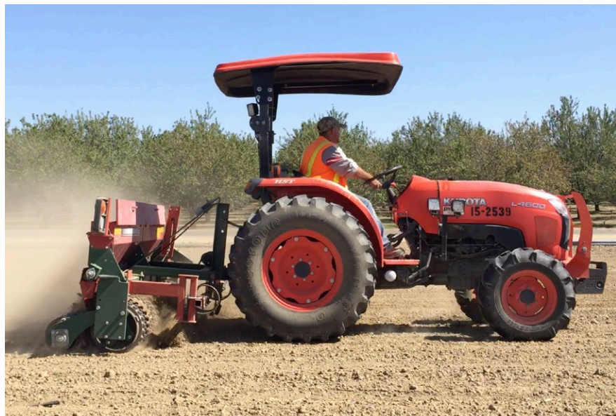
Seeding a wildflower planting with a mechanical drop seeder and cultipacker. Photograph: Katharina Ullmann, The Xerces Society.
