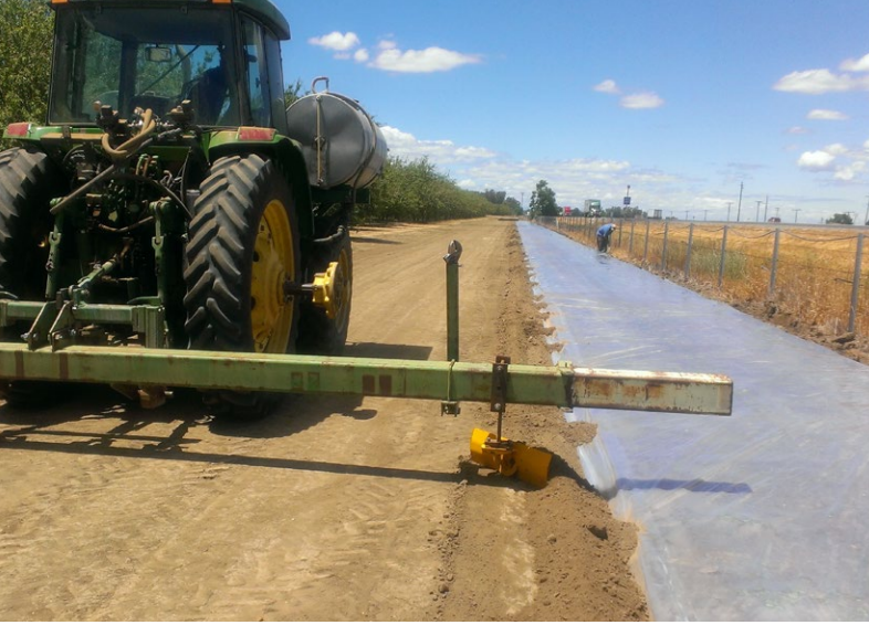
Burying the edges of solarization plastic using a bar-mounted trenching implement. Photograph: Jessa Kay Cruz, The Xerces Society.
