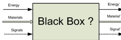
Fig 5. The conversion of energy, material and signals. Solution not yet known; task or function described on the basis of inputs and outputs, Pahl and Beitz[8]
