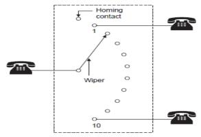
The contact arm (wiper) moves across a fixed set of switch contacts. In the case single uniselector, each contact is connected to an outgoing channel, so a caller can choose to connect to any of 10 different subscribers by dialling any digit from 1 to 10. As this selector moves in just one plane, thus sort of automated selector is known as uniselector.
