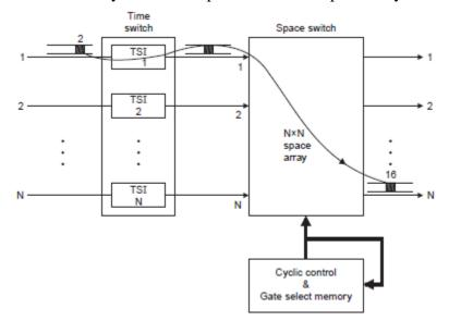
The transmission of signals carried out from sender to receiver through multiplexer input and de multiplexer output. The reverse communication also similar. Thus a hybrid arrangement is needed to isolate the transmitted signal from the received signal. The basic function of the time switch is to delay information in arriving time slots until the desired output time slot occurs.
