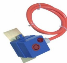
Fig 3 Temperature sensor (LM35)
