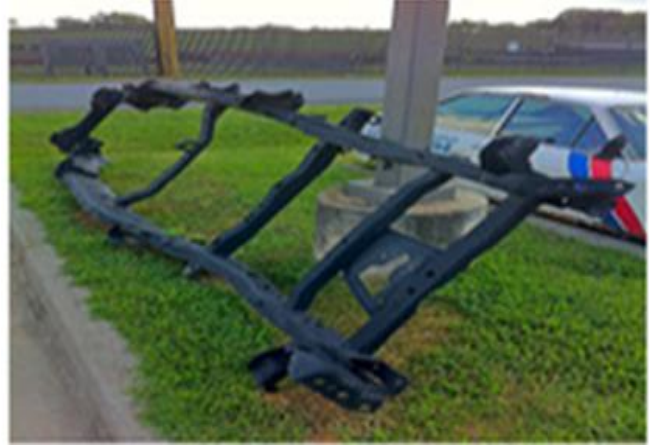
Fig.2. A Bare Ladder Frame
