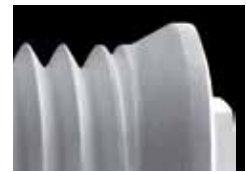
50X photo scanning of BT EVO DL SP implant profile
