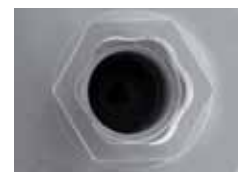
Photo scanning (50X) external hexagon connection
