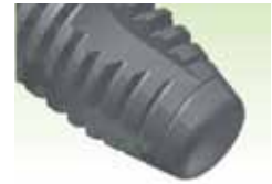
The flaring of the passage from the head to the body of the implant can be used, at the operator's discretion, to be positioned at a crestal or sub-crestal level, thereby enabling to obtain great primary stability even in poor quality bone.
