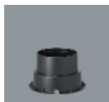
33961.000 Housing for recessed mounting Corrosion-resistant cast aluminium, No-Rinse surface treatment. Black double powder-coated. 2 cable entries. Weight 3.80kg
