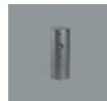
34958.000 Adapter sleeve for poles ø 76mm and cantilever arms. Housing and cover: corrosion-resistant cast aluminium, No-Rinse surface treatment. Graphit m, double powder- coated. Screw fixing. Terminal block 5x2,5mm 2 . Through- wiring possible. 2 cable entries for cantilever arms. Protection mode IP44 only with ac- cessories. Cantilever arms to be ordered separ- ately. Poles ø 76mm to be ordered separately. Weight 3.80kg
