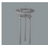
33980.000 Concrete anchor Mounting plate with threaded bar and fixing nuts M6. Individual parts to be assembled on-site. Weight 0.30kg
