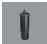
34974.000 Distribution box, IP68 With four cable entries, 7-25mm. Plastic. ø 102mm, L 305mm. Weight 0.47kg
