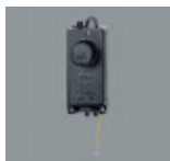
34964.000 Cable junction box, IP54 Plastic, black. Terminal block 2 of 5x2.5mm 2 . 1 fuse D01 E14 10A. Weight 0.25kg
