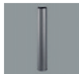
34963.000 Post for adapter sleeves. Metal, hot-dip galvanised. Graphit m, double powder-coated. Mounting plate: metal. 5-pole terminal block for cable 5x2.5mm 2 . Through-wiring possible. IP44 protection mode when used with relevant accessories. Not for concrete anchor 33980.000 and mounting plate 33982.000. Weight 1.50kg
