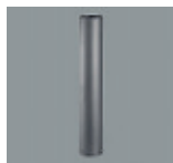
34962.000 Post Metal, hot-dip galvanised. Graphit m, double powder-coated. Mounting plate: metal. 5-pole terminal block for cable 5x2.5mm 2 . Through-wiring possible. 3-pole terminal block for control line. Luminaire rotatable through 360°. Protection mode IP44 in connection with mounted luminaire. Weight 5.60kg
