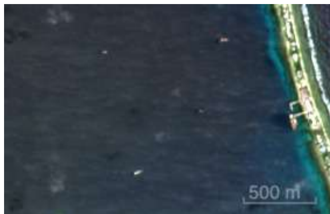
Figure 3a: Vessels visible in 10 m resolution data from the Sentinel-2 satellite in Funafuti lagoon, Tuvalu, from 27 March 2021. The image swath has a width of 290 km. The four vessels visible in the lagoon have a length of 30 m or longer.
