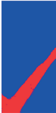
Figure 7-9: Localized damaged zone inside the sample. Blue color represents undamaged part and red damage above 5%. The thickness of the damaged area represents an internal characteristic length for the FE-tunnel application.
