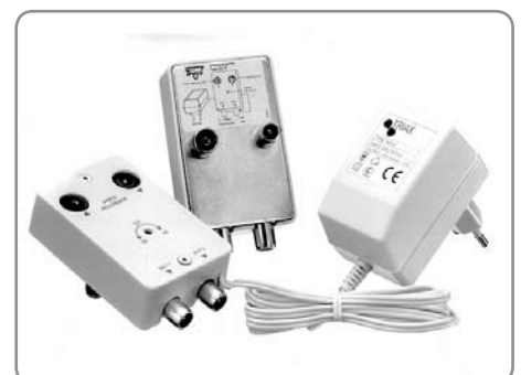
2TVplus amplifiers for mounting directly on the outlet box
