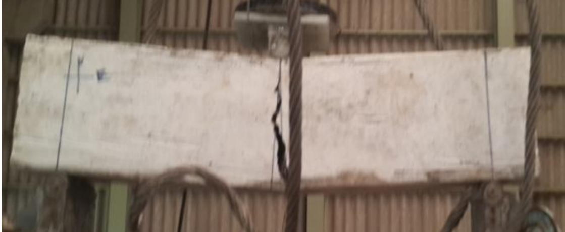
Plate 4.12: Failure pattern of Steel 101 beam
