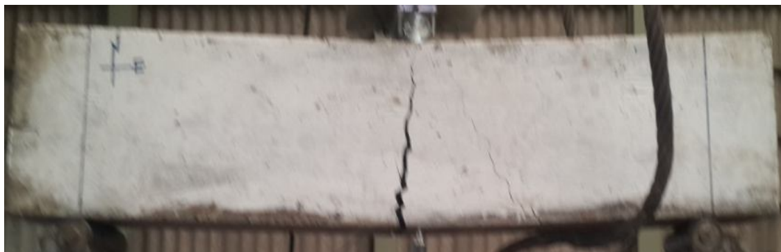
Plate 4.6: Failure pattern of L.B.805 beam
