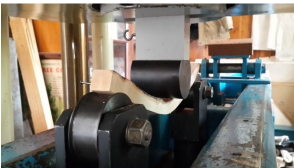
Plate 4.2: Beam test specimen under loading
