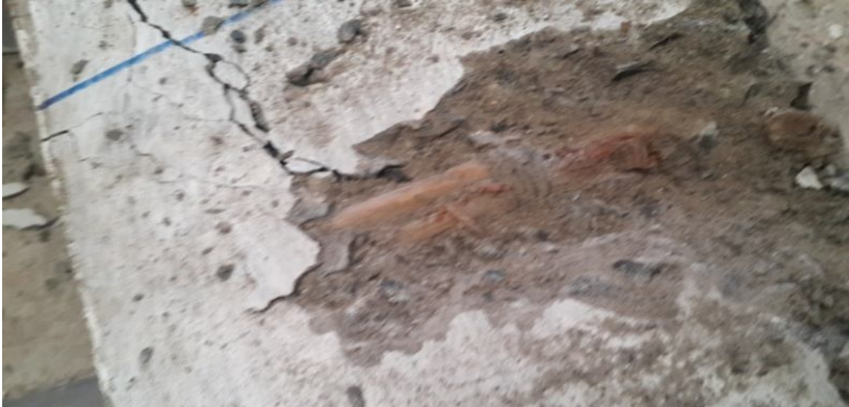
Plate 4.17: unbroken shear reinforcement for L.B.2x10 beam
