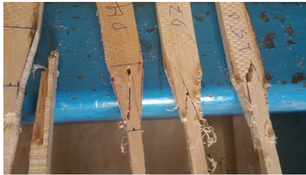
Plate 4.1: Tensile test samples mode of failure
