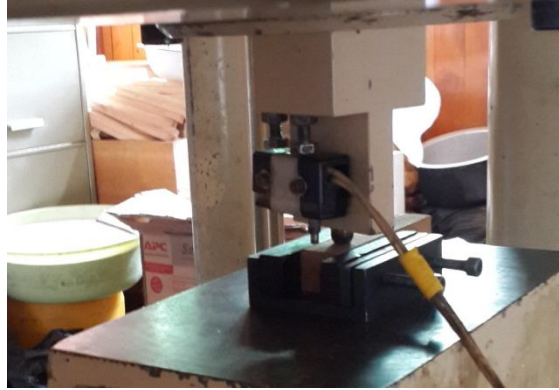
Plate 3.5: Janka hardness test
