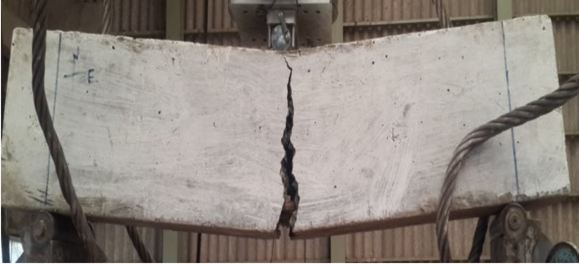
Plate 4.10: Failure pattern of L.B.419 beam
