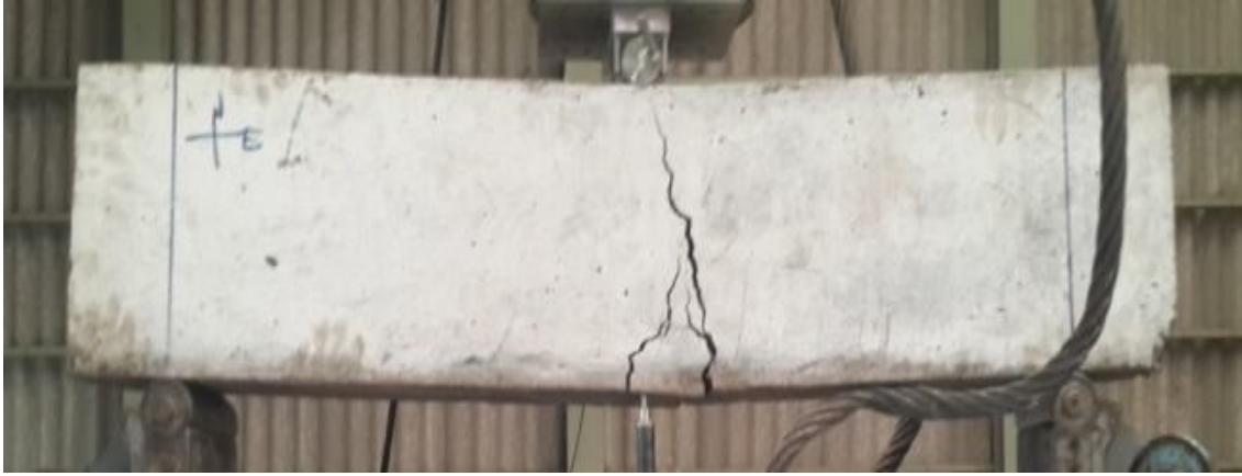
Plate 4.8: Failure pattern of L.B.741 beam
