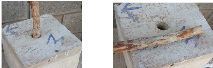
Plate 4.4: Mode of interfacial bond failure of L. buchananii in concrete
