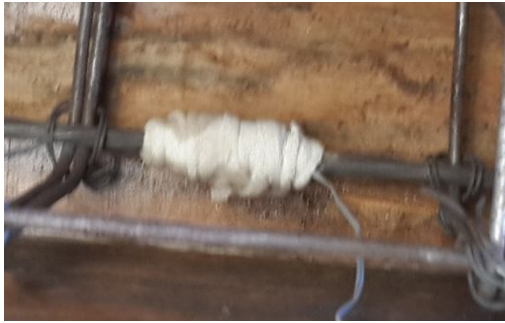
Plate 3.12: Covered/bandaged strain gauge
