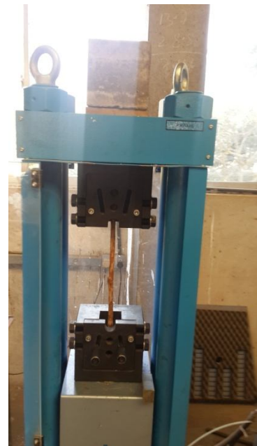
Plate 3.7: Pull out test
