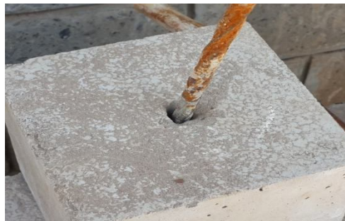
Plate 4.5: Mode of interfacial bond failure of steel in concrete
