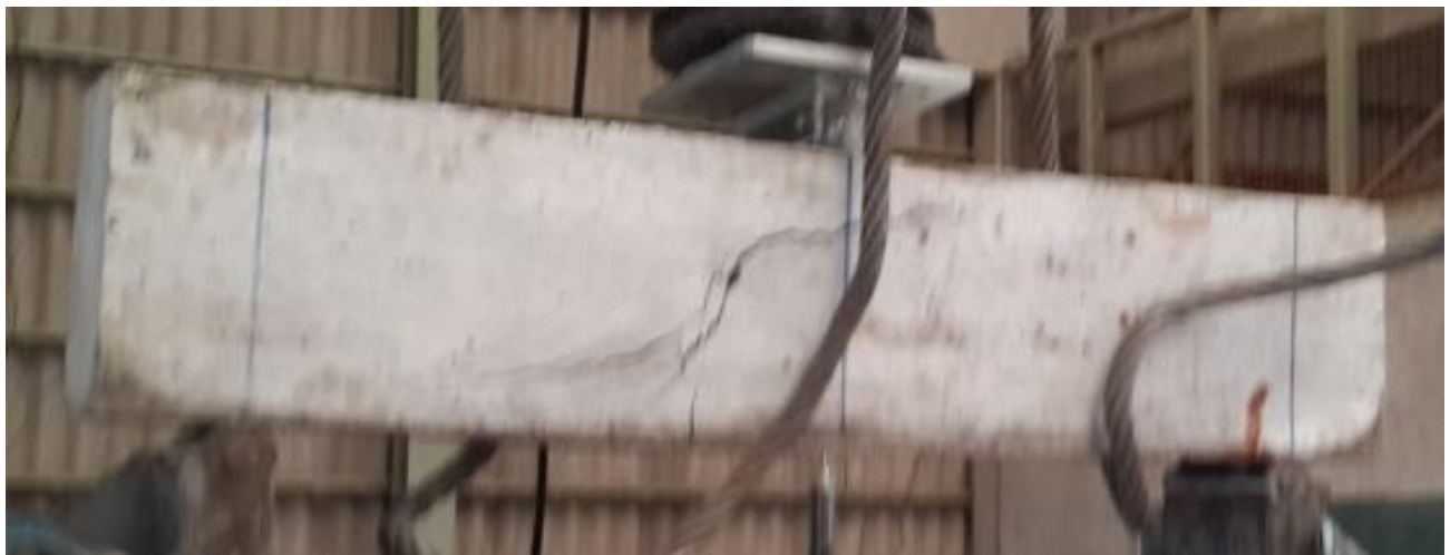
Plate 4.20: Failure pattern of L.B.2x13 beam
