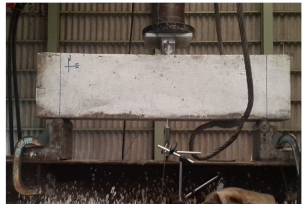
Plate 3.17: Beam set up for testing
