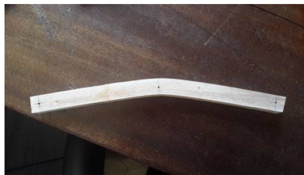
Plate 4.3: Beam test sample after loading
