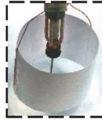
Fig. 1. Transducer probe mounted in a hollow cardboard cylinder of 1-cm radius and 2-cm height.
