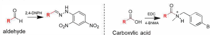
Figure 1. Derivatization of aldehydes with 2,4-DNPH and carboxylic acids with 4-BNMA coupled with EDC.
