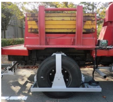
Fig. 1 Installation state of deck for sensor
