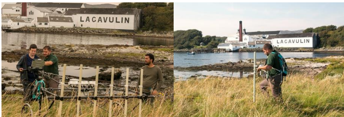
Figure 11 Bartington magnetic cart with six sensors and the hand-held dual sensor magnetic gradiometer during 2019 survey at Dunyvaig.
