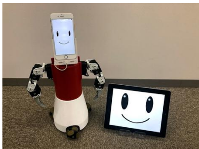
Fig.5 Robot partner equipped with moving mechanism
