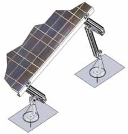
Weather-tight flashing and standoffs for tilt applications
