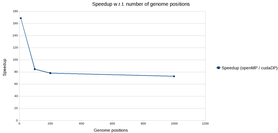
Figure 1. Speedup of GPU-QTLMap / OpenMP-QTLMap (8 cores) over the number of genome positions
